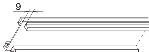
transom cut-out the base
